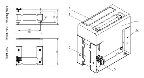
**Description: 1**/ epoxy resin casting, **2**/ core (UNICORE), **3**/ fuse + upper voltage terminal, **4**/ insulating guard made of silicone rubber, **5**/ lower voltage terminals; terminal blocks **16** or **6** mm<sup>2</sup>, **6**/ housing
